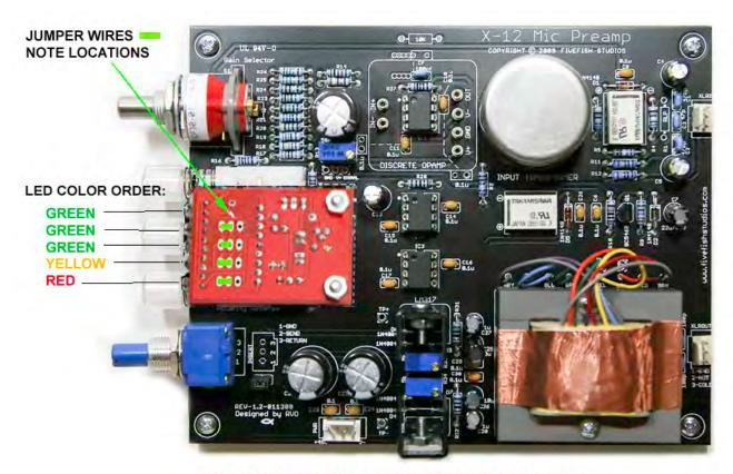
NOTE: VU METER BOARD IS INSTALLED UPSIDE DOWN
