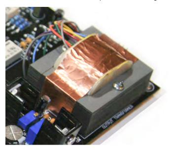
NOTE: You may want to do STEP 13 LAST, after adjusting the voltages on the X-12 board. This is to prevent damage to the IC chips in case the voltage is too high before adjustments.
