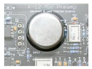
ERRATA: Short pins 1-2, and 3-4 at bottom of PCB.
