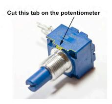
IMPORTANT: Make sure you cut/snip the tab located on one side of the blue potentiometer. Cutting this tab will make the potentiometer stay straight and perpendicular to the Front Panel as you tighten the nut.
