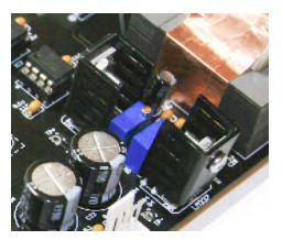
STEP 11: Install the Input Transformer. For the Input Transformer, orient the "dot" with the printed silkscreen dot on the PCB. Don't forget to also install the R2/RLS resistor located on the lower left corner of the Input Transformer.
