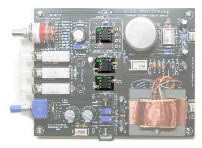
Above is a photo showing the locations of IC1, IC2 and IC3. Note the proper orientation of the chips.
