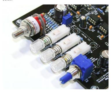
Some boutique preamp manufacturers also use Grayhill selector switches for their preamps. They are durable, reliable, have a nice solid feel to it, and provide good resistance to RF Interference. This switch will be the most commonly used/abused mechanical device on the X-12 preamp. I want this part to withstand being turned and turned and turned and is just one of the expensive parts in this kit.
