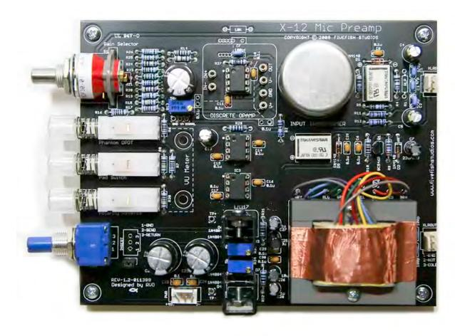
The general guideline in electronics assembly is to solder the smallest/shortest component first (resistors, diodes, inductors), and solder the bigger/taller components last (ceramic capacitors, electrolytic capacitors, switches, etc).
