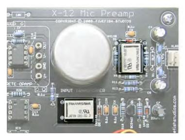
Also make sure the Relay is oriented in the correct direction. Follow the "line marking" on the component with the printed silkscreen on the board.
